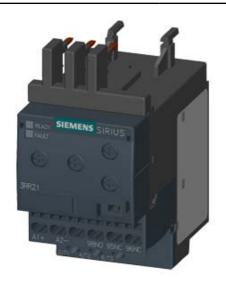
MONITORING RELAY ATTACHABLE TO CONTACTOR 3RT2. SIZE S00 BASIC, ANALOG ADJUSTABLE APPARENT CURRENT MONITORING 1.6 - 16A, 50-60 HZ, 2-PHASE SUPPLY 24 V AC/DC 1 CO CONTACT MONITORING FOR CURRENT OVERSHOOT/UNDERSHOOT PHASE FAILURE, WIRE BREAK WITH OR W/O ERROR LOG ON-DELAY 0-60 S SPURIOUS PEAK SUPPR.0-30 S SWITCHING HYSTERESIS 6% SPRING-LOADED CONNECTION
