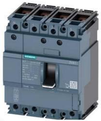
CIRCUIT BREAKER 3VA1 IEC FRAME 100 BREAKING CAPACITY CLASS B ICU=16KA @ 415 V 4-POLE, LINE PROTECTION TM210, FTFM, IN=16A OVERLOAD PROTECTION IR=16A FIXED SHORT CIRCUIT PROTECTION II=10 X IN NEUTRAL UNPROTECTED BUSBAR CONNECTION
