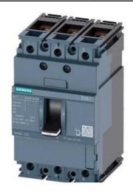
CIRCUIT BREAKER 3VA1 IEC FRAME 100 BREAKING CAPACITY CLASS N ICU=25KA @ 415 V 3-POLE, LINE PROTECTION TM210, FTFM, IN=16A OVERLOAD PROTECTION IR=16A FIXED SHORT CIRCUIT PROTECTION II=10 X IN BUSBAR CONNECTION
