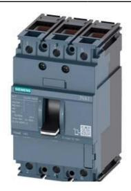
CIRCUIT BREAKER 3VA1 IEC FRAME 160 BREAKING CAPACITY CLASS N ICU=25KA @ 415 V 3-POLE, LINE PROTECTION TM210, FTFM, IN=125A OVERLOAD PROTECTION IR=125A FIXED SHORT CIRCUIT PROTECTION II=10 X IN CABLE CONNECTION
