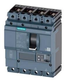
CIRCUIT BREAKER 3VA2 IEC FRAME 160 BREAKING CAPACITY CLASS L ICU=150KA @ 415 V 4POLE, LINE PROTECTION ETU550, LSI, IN=160A OVERLOAD PROTECTION IR=64A ...160A SHORT CIRCUIT PROTECTION ISD=0,6..10X IN, II=1,5..10X IN NEUTRAL PROTECTION ADJUSTABLE (OFF, UPTO 100%) BUSBAR CONNECTION
