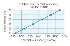
Thermally Conductive, Reinforced Gap Filling Material
