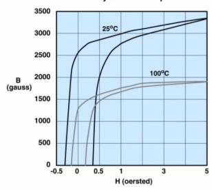
Measured on a 17/10/6mm toroid at 10kHz.
