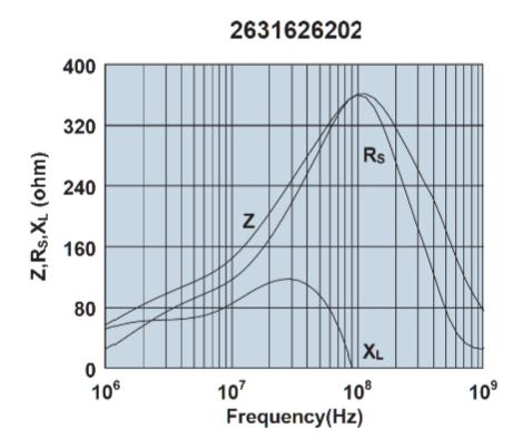
Impedance, reactance, and resistance vs. frequency.
