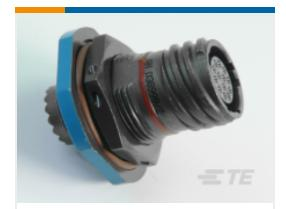
TE Part #YDTS24Z21-16SAV001 Jam Nut: D38999, 21-16 Insert, Black Zinc Nickel Plating
