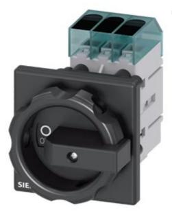
Switch disconnector 3LD3, main switch 3-polig, lu 16A operational switch at AC-23 A at 400 V 7,5 kW front mounted Base mounting with center-hole 22,5 mm rotary operationg mechanism black 66 x66 mm
