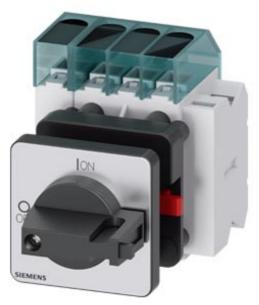
Switch disconnector 3LD3, main switch 3-polig + N, lu 63A operational switch at AC-23 A at 400 V 22,0 kW front mounted Base mounting with center-hole 22,5 mm knob-operated mechanism black  $48 \times 48$  mm with auxiliary 1NO+1NC
