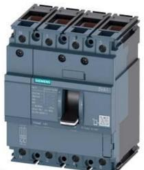
CIRCUIT BREAKER 3VA1 IEC FRAME 160 BREAKING CAPACITY CLASS S ICU=36KA @ 415 V 4-POLE, LINE PROTECTION TM210, FTFM, IN=100A OVERLOAD PROTECTION IR=100A FIXED SHORT CIRCUIT PROTECTION II=10 X IN NEUTRAL PROTECTION 100% CABLE CONNECTION
