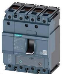
CIRCUIT BREAKER 3VA1 IEC FRAME 160 BREAKING CAPACITY CLASS N ICU=25KA @ 415 V 4-POLE, LINE PROTECTION TM240, ATAM, IN=50A OVERLOAD PROTECTION IR=35A ...50A SHORT CIRCUIT PROTECTION II=5...10 X IN NEUTRAL PROTECTION 100% CABLE CONNECTION
