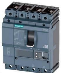
CIRCUIT BREAKER 3VA2 IEC FRAME 100 BREAKING CAPACITY CLASS L ICU=150KA @ 415 V 4POLE, LINE PROTECTION ETU550, LSI, IN=40A OVERLOAD PROTECTION IR=16A ...40A SHORT CIRCUIT PROTECTION ISD=0,6..10X IN, II=1,5..12X IN NEUTRAL PROTECTION ADJUSTABLE (OFF, UPTO 160%) BUSBAR CONNECTION
