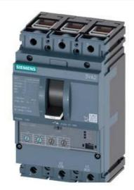
CIRCUIT BREAKER 3VA2 IEC FRAME 100 BREAKING CAPACITY CLASS L ICU=150KA @ 415 V 3POLE, LINE PROTECTION ETU330, LIG, IN=63A OVERLOAD PROTECTION IR=25A ...63A SHORT CIRCUIT PROTECTION II=1,5...12 X IN GROUNDFAULTPROTECTION IG=0,2... 1 X IN, TG=0,1/0,3MS CABLE CONNECTION
