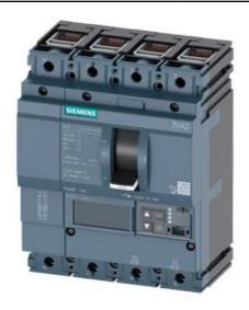
CIRCUIT BREAKER 3VA2 IEC FRAME 160 BREAKING CAPACITY CLASS C ICU=110KA @ 415 V 4POLE, LINE PROTECTION ETU560, LSIG, IN=63A OVERLOAD PROTECTION IR=25A ...63A SHORT CIRCUIT PROTECTION ISD=0,6..10X IN, II=1,5..12X IN NEUTRAL PROTECTION ADJUSTABLE (OFF, UPTO 160%) GROUNDFAULT, SWITCHABLE IG=0,2... 1 X IN, TG=0,050,8MS CABLE CONNECTION
