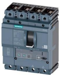
CIRCUIT BREAKER 3VA2 IEC FRAME 250 BREAKING CAPACITY CLASS M ICU=55KA @ 415 V 4POLE, LINE PROTECTION ETU320, LI, IN=160A OVERLOAD PROTECTION IR=64A ...160A SHORT CIRCUIT PROTECTION II=12 X IN NEUTRAL PROTECTION ADJUSTABLE(OFF,50%,100%) BUSBAR CONNECTION
