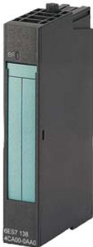
SIMATIC DP, ELECTRONIC MODULE FOR ET200S, 2 AO U HIGH SPEED, 15 MM WIDTH, +/-10V, +/-5V, 1.. 5V; 16BIT, CYCLE TIME: 0.1 MS WITH LED SF (GROUP FAULT)
