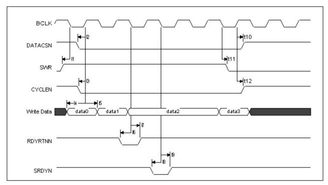
Figure 16. Synchronous Burst Write Cycles – VLBUSN = 1
