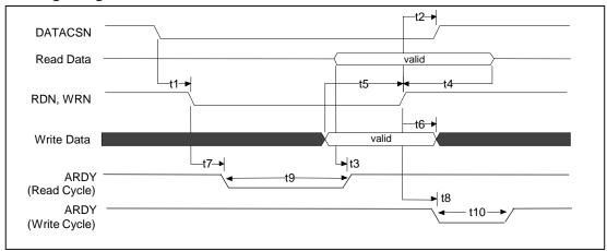
Figure 14. Asynchronous Cycle – Using DATACSN
