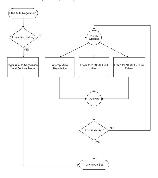
Figure 8. Auto Negotiation and Parallel Operation
