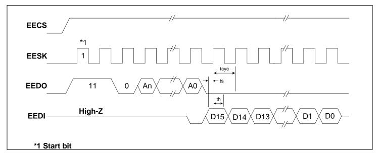
Figure 22. EEPROM Read Cycle Timing Diagram
