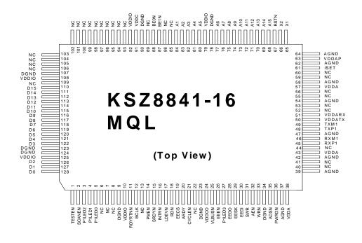
Figure 2. Standard – KSZ8841-16 MQL 128-Pin PQFP (Top View)
