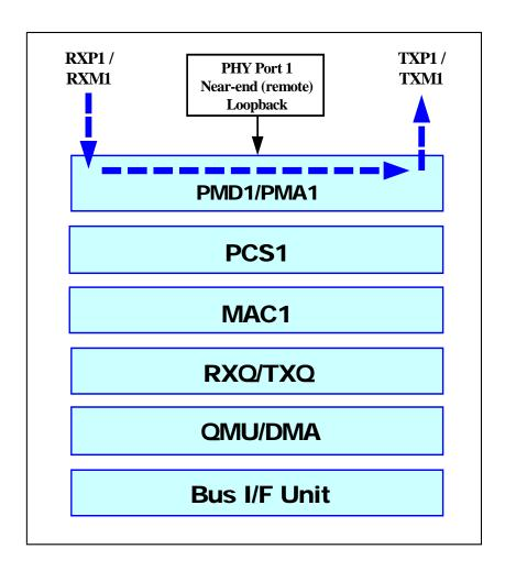
Figure 11. PHY Port 1 Near-end (Remote) Loopback Path
