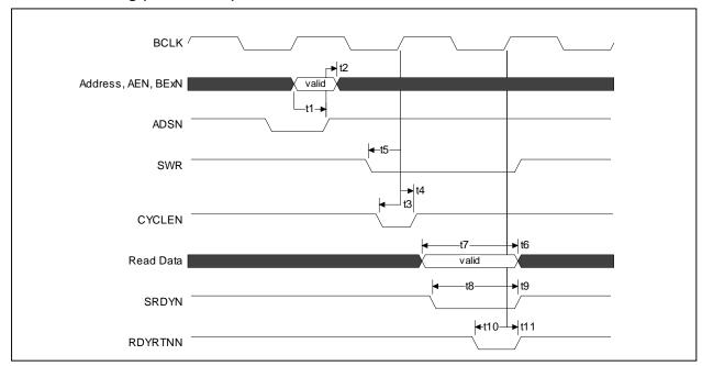
Figure 19. Synchronous Read Cycle – VLBUSN = 0
