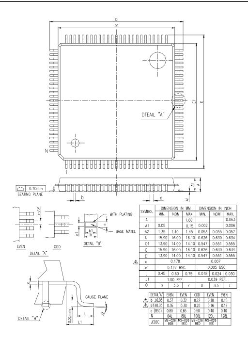
Figure 24. Optional 128-Pin LQFP Package
