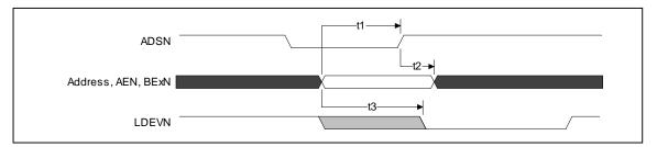
Figure 15. Address Latching Cycle for All Modes
