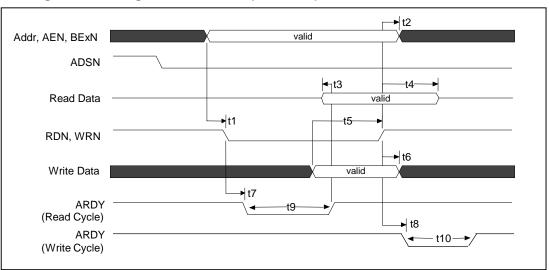
Figure 12. Asynchronous Cycle – ADSN = 0
