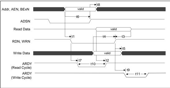
Figure 13. Asynchronous Cycle - Using ADSN
