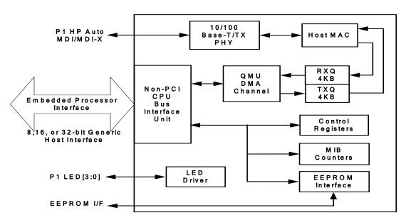
Figure 1. KSZ8841M Functional Diagram
