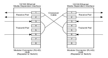
Figure 7. Typical Crossover Cable Connection
