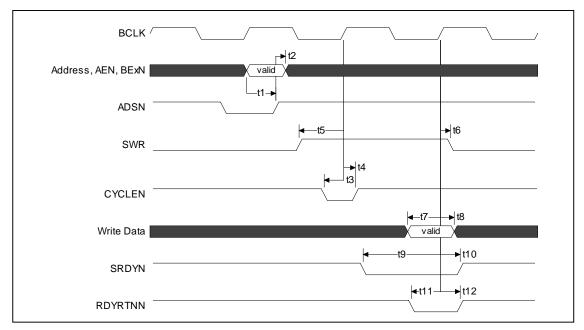
Figure 18. Synchronous Write Cycle – VLBUSN = 0
