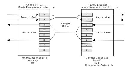
Figure 6. Typical Straight Cable Connection
