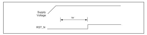
Figure 21. Reset Timing
