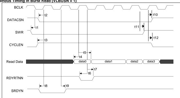
Synchronous Timing in Burst Read (VLBUSN = 1)
