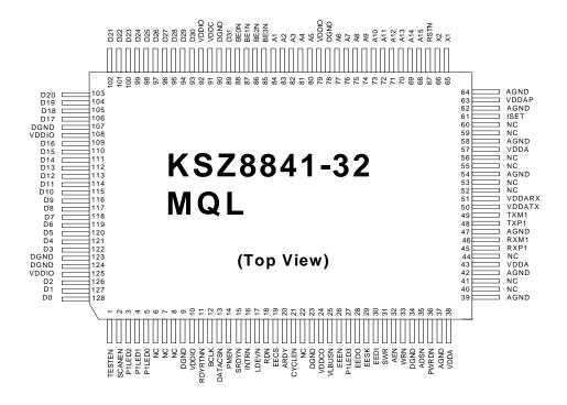
Figure 4. Standard – KSZ8841-32 MQL 128-Pin PQFP (Top View)
