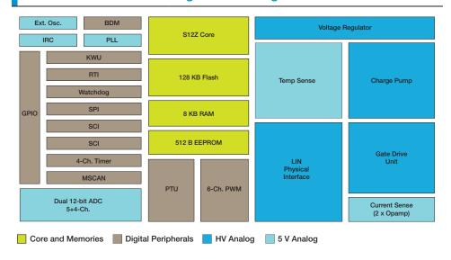
The MC9S12ZVML128 is part of the S12 MagniV portfolio of mixed-signal MCUs, offering smart and optimized integration of high-voltage analog components. The MC9S12ZVML128 product family integrates an automotive voltage regulator operating between 3.5 and 40 volts, a LIN physical layer and a gate drive unit made of three low-side and three high-side drivers to control up to six external MOSFETs.
