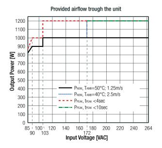
The units were evaluated to safety files for nominal input voltages 100-240VAC; including a tolerance band of  $\pm 10\%$ , with a specified maximum  $T_{BASE}$  of 80°C for full load rating with 50°C  $T_{AMB}$  and up to 80°C  $T_{AMB}$ . at reduced output power.  $T_{BASE}$  at reference point (see "thermal reference point") shall not exceed 70°C, 80°C or 90°C depending on the condition as per derating graph.
