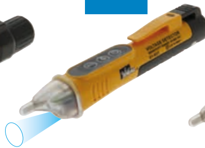
61-637 Single Range 24 to 600V AC NCVT w/Torch CAT IV 600V
