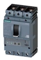
circuit breaker 3VA2 IEC frame 160 breaking capacity class E Icu=200 kA @ 415 V 3-pole, line protection ETU330, LIG, In=100A overload protection Ir=40A ... 100A short circuit protection Ii=1,5...12 x In ground fault protection Ig=0,2... 1 x In, tg=0,1/0,3s busbar connection
