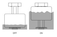
When mounted near ferromagnetic parts switching distance of RND 410-00003 may vary  $\,$
