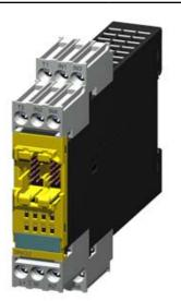
SIRIUS, EXPANSION MODULE 3RK32 FOR MODULAR SAFETY SYSTEM 3RK3 2/4 F-DI, 2 F-DO, 24V DC/1.2A PARAMETERIZABLE VIA SW MSS ES WIDTH 22.5MM SCREW TERMINAL UP TO SIL3 (IEC 61508) UP TO PERFORMANCE LEVEL E (ISO 13849-1)
