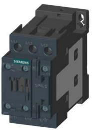
CONTACTOR, AC-3, 11KW/400V, 1NO+1NC, DC 24V, W.INTEGR.DIODE 3-POLE, SZ S0 SCREW TERMINAL
