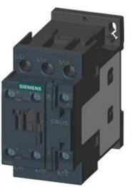
CONTACTOR, AC-3, 18.5KW/400V, 1NO+1NC, AC 42V 50HZ, 3-POLE, SZ S0 SCREW TERMINAL
