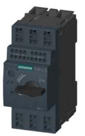
CIRCUIT-BREAKER SZ S00, FOR MOTOR PROTECTION, CLASS 10, A-REL.1.8...2.5A, N-RELEASE 33A, SPRING-L. CONNECTION, STANDARD SW. CAPACITY W. TRANSVERSE AUX. SWITCH 1NO+1NC
