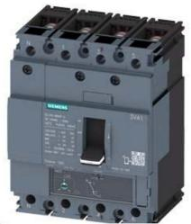
CIRCUIT BREAKER 3VA1 IEC FRAME 160 BREAKING CAPACITY CLASS H ICU=70KA @ 415 V 4-POLE, LINE PROTECTION TM220, ATFM, IN=100A OVERLOAD PROTECTION IR=70A ...100A SHORT CIRCUIT PROTECTION II=10 X IN NEUTRAL PROTECTION 50% BUSBAR CONNECTION
