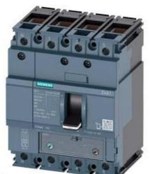
CIRCUIT BREAKER 3VA1 IEC FRAME 160 BREAKING CAPACITY CLASS H ICU=70KA @ 415 V 4-POLE, LINE PROTECTION TM240, ATAM, IN=100A OVERLOAD PROTECTION IR=70A ...100A SHORT CIRCUIT PROTECTION II=5...10 X IN NEUTRAL PROTECTION 100% CABLE CONNECTION
