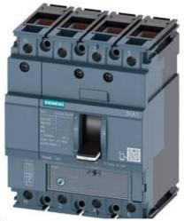
CIRCUIT BREAKER 3VA1 IEC FRAME 160 BREAKING CAPACITY CLASS S ICU=36KA @ 415 V 4-POLE, LINE PROTECTION TM220, ATFM, IN=20A OVERLOAD PROTECTION IR=14A ...20A SHORT CIRCUIT PROTECTION II=10 X IN NEUTRAL UNPROTECTED CABLE CONNECTION
