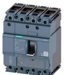
CIRCUIT BREAKER 3VA1 IEC FRAME 160 BREAKING CAPACITY CLASS H ICU=70KA @ 415 V 4-POLE, LINE PROTECTION TM220, ATFM, IN=32A OVERLOAD PROTECTION IR=22,4A ...32A SHORT CIRCUIT PROTECTION II=10 X IN NEUTRAL UNPROTECTED BUSBAR CONNECTION
