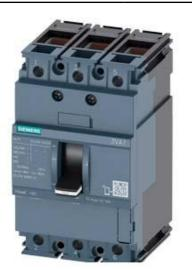
CIRCUIT BREAKER 3VA1 IEC FRAME 160 BREAKING CAPACITY CLASS N ICU=25KA @ 415 V 3-POLE, LINE PROTECTION TM210, FTFM, IN=40A OVERLOAD PROTECTION IR=40A FIXED SHORT CIRCUIT PROTECTION II=10 X IN CABLE CONNECTION
