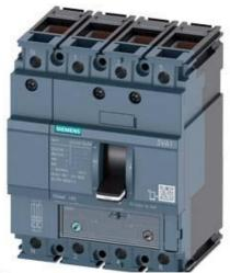
CIRCUIT BREAKER 3VA1 IEC FRAME 160 BREAKING CAPACITY CLASS S ICU=36KA @ 415 V 4-POLE, LINE PROTECTION TM240, ATAM, IN=40A OVERLOAD PROTECTION IR=28A ...40A SHORT CIRCUIT PROTECTION II=5...10 X IN NEUTRAL PROTECTION 100% CABLE CONNECTION
