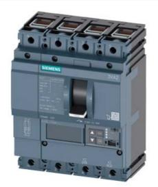
CIRCUIT BREAKER 3VA2 IEC FRAME 100 BREAKING CAPACITY CLASS M ICU=55KA @ 415 V 4POLE, LINE PROTECTION ETU860, LSIG, IN=100A OVERLOAD PROTECTION IR=40A ...100A SHORT CIRCUIT PROTECTION ISD=0,6..10X IN, II=1,5..12X IN NEUTRAL PROTECTION ADJUSTABLE (OFF, UPTO 100%) GROUNDFAULT, SWITCHABLE IG=0,2... 1 X IN, TG=0,050,8MS CABLE CONNECTION
