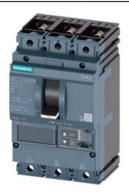
CIRCUIT BREAKER 3VA2 IEC FRAME 100 BREAKING CAPACITY CLASS H ICU=85KA @ 415 V 3POLE, LINE PROTECTION ETU560, LSIG, IN=25A OVERLOAD PROTECTION IR=10A ...25A SHORT CIRCUIT PROTECTION ISD=0,6..10X IN, II=1,5..12X IN NEUTRAL PROTECTION OPTIONAL WITH EXT. CT,UPTO 160% GROUNDFAULT, SWITCHABLE IG=0,2... 1 X IN, TG=0,050,8MS BUSBAR CONNECTION
