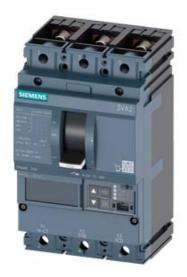
CIRCUIT BREAKER 3VA2 IEC FRAME 250 BREAKING CAPACITY CLASS M ICU=55KA @ 415 V 3POLE, LINE PROTECTION ETU550, LSI, IN=160A OVERLOAD PROTECTION IR=64A ...160A SHORT CIRCUIT PROTECTION ISD=0,6..10X IN, II=1,5..12X IN NEUTRAL PROTECTION OPTIONAL WITH EXT. CT,UPTO 160% BUSBAR CONNECTION
