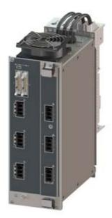
SIPLUS HCS4300 POM4320 Busbar Mounting (UL). Power Output Module for mounting on power rail system. Redesign with increased EMC resistance. With 9 power outputs each max.7200 W (with control mode half-wave control: Depending on the inrush current of the electric load there is a limitation of max. 4000 W)
