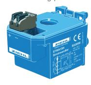
The STWA1SH has an integrated electronic with transistor-output. The switching point is 2A. Above app. 2 A the output transistor is switched on below app. 1.5 A it is off.
