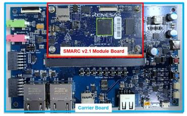
Evaluate both RISC-V CPU and Arm CPU by replacing <u>SMARC module for RZ/Five (RISC-V)</u> and <u>SMARC module for RZ/G2UL (Arm)</u> on the carrier board.
