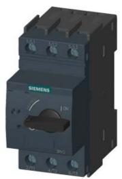
CIRCUIT-BREAKER SZ S0, FOR STARTER COMBINATION, RATED CURRENT 32A, N-RELEASE 400A, SCREW CONNECTION, STANDARD SW. CAPACITY
