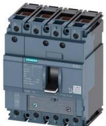
CIRCUIT BREAKER 3VA1 IEC FRAME 160 BREAKING CAPACITY CLASS S ICU=36KA @ 415 V 4-POLE, LINE PROTECTION TM240, ATAM, IN=63A OVERLOAD PROTECTION IR=44,1A ...63A SHORT CIRCUIT PROTECTION II=5...10 X IN NEUTRAL UNPROTECTED CABLE CONNECTION
