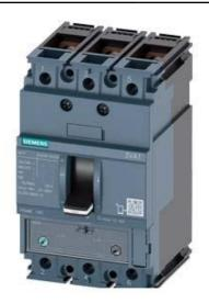
CIRCUIT BREAKER 3VA1 IEC FRAME 160 BREAKING CAPACITY CLASS N ICU=25KA @ 415 V 3-POLE, LINE PROTECTION TM240, ATAM, IN=80A OVERLOAD PROTECTION IR=56A ...80A SHORT CIRCUIT PROTECTION II=5...10 X IN BUSBAR CONNECTION
