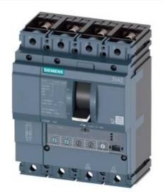
CIRCUIT BREAKER 3VA2 IEC FRAME 160 BREAKING CAPACITY CLASS C ICU=110KA @ 415 V 4POLE, LINE PROTECTION ETU350, LSI, IN=160A OVERLOAD PROTECTION IR=64A ...160A SHORT CIRCUIT PROTECTION ISD=1,5... 10 X IR, II=10 X IN NEUTRAL PROTECTION ADJUSTABLE(OFF,50%,100%) BUSBAR CONNECTION
