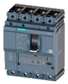
CIRCUIT BREAKER 3VA2 IEC FRAME 160 BREAKING CAPACITY CLASS C ICU=110KA @ 415 V 4POLE, LINE PROTECTION ETU350, LSI, IN=40A OVERLOAD PROTECTION IR=16A ...40A SHORT CIRCUIT PROTECTION ISD=1,5... 10 X IR, II=12 X IN NEUTRAL PROTECTION ADJUSTABLE(OFF,100%) BUSBAR CONNECTION
