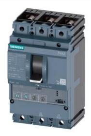
CIRCUIT BREAKER 3VA2 IEC FRAME 250 BREAKING CAPACITY CLASS C ICU=110KA @ 415 V 3POLE, LINE PROTECTION ETU350, LSI, IN=160A OVERLOAD PROTECTION IR=64A ...160A SHORT CIRCUIT PROTECTION ISD=1,5... 10 X IR, II=12 X IN BUSBAR CONNECTION
