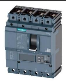
CIRCUIT BREAKER 3VA2 IEC FRAME 250 BREAKING CAPACITY CLASS H ICU=85KA @ 415 V 4POLE, LINE PROTECTION ETU860, LSIG, IN=250A OVERLOAD PROTECTION IR=100A ...250A SHORT CIRCUIT PROTECTION ISD=0,6..10X IN, II=1,5..10X IN NEUTRAL PROTECTION ADJUSTABLE (OFF, UPTO 100%) GROUNDFAULT, SWITCHABLE IG=0,2... 1 X IN, TG=0,050,8MS BUSBAR CONNECTION
