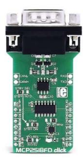
The physical layer is implemented by using a separate IC, which provides increased robustness, required for the automotive applications. It features three operating modes,
