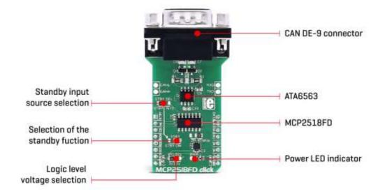
The role of the CAN bus controller is to provide arbitration, message framing, message validation, error detection, message filtering, and so on. Among all other tasks - it is used to provide clearly formatted CAN data for the application layer, running on the host MCU.
