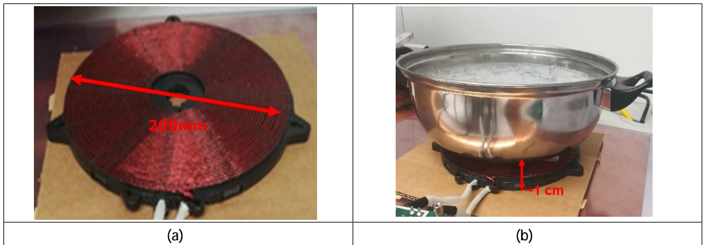
Figure 18 Picture of the resonant coil (a) and positioning of the cooking vessel (b)
