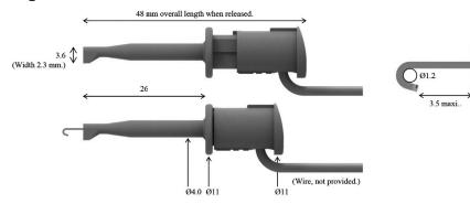
The hook fits to 1.2mm diameter round pins and 0.9mm × 0.9mm square pins. The gold plating prevents oxidation and keeps good electrical conductance.
