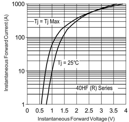
Fig. 12 - Forward Voltage Drop Characteristics (For 1400 V/1600 V)
