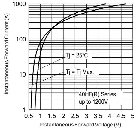
Fig. 11 - Forward Voltage Drop Characteristics (Up To 1200 V)
